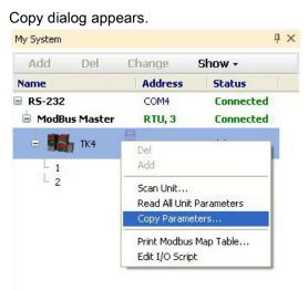
4th Right-click the unit which parameters are saved and select 'Parameter Select'. The parameter values of the unit is loaded at the right side of the dialog.
